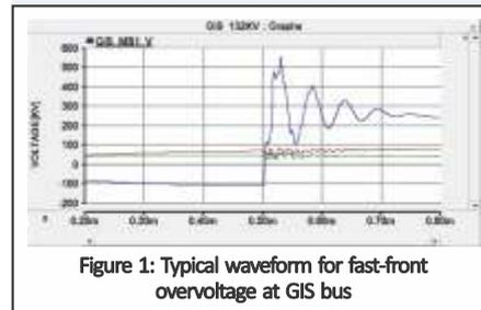
Figure 1: Typical waveform for fast-front overvoltage at GIS bus
