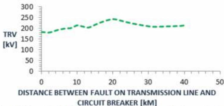
Figure 3: Magnitude of TRV vs. Location of fault on the transmission line
