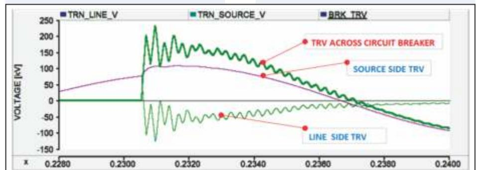
Figure 1: Transient recovery voltage for transmission line fault [1<sup>st</sup> pole clearance]
