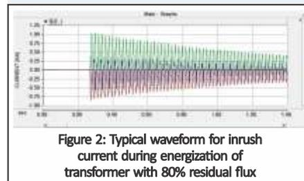
Figure 2: Typical waveform for inrush current during energization of transformer with 80% residual flux
