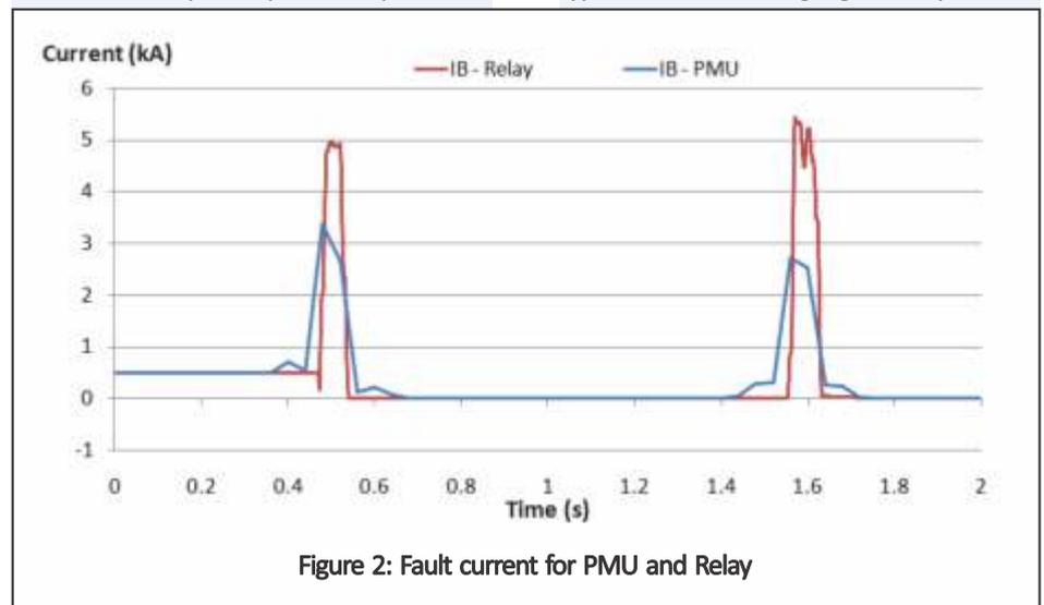
Figure 2: Fault current for PMU and Relay
