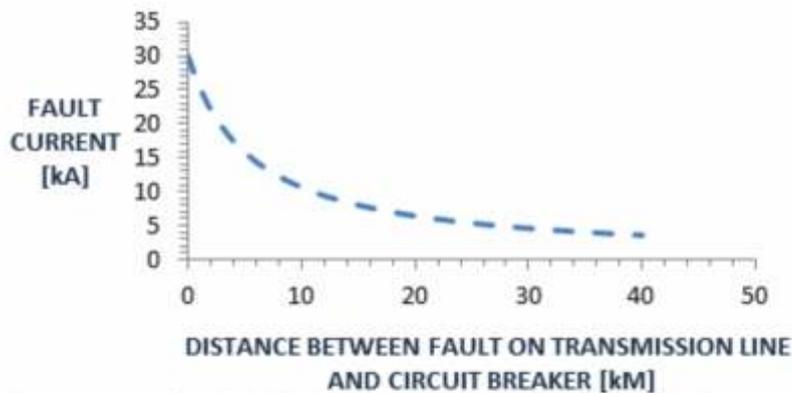
Figure 2: Magnitude of fault current vs. Location of fault on the transmission line
