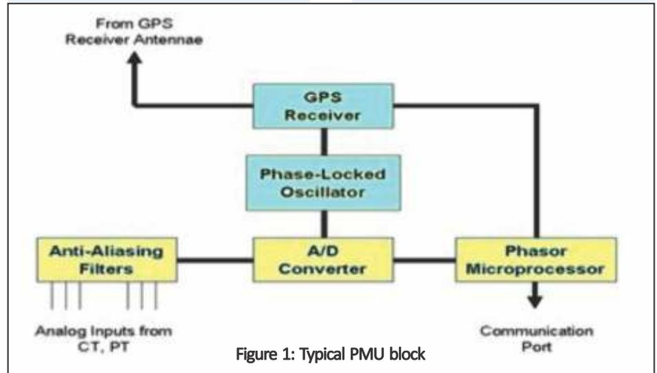
Figure 1: Typical PMU block
