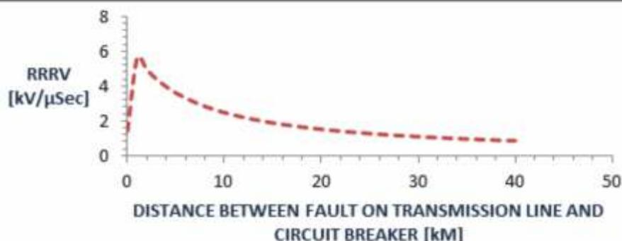
Figure 4: Magnitude of RRRV vs. Location of fault on the transmission line
